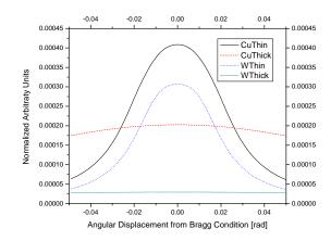
Fig. 1. W222 and Cu111 crystal theoretical PXR photon distribution broadening for 1-mm thick crystals compared to thin crystals optimized for 15 KeV PXR.
