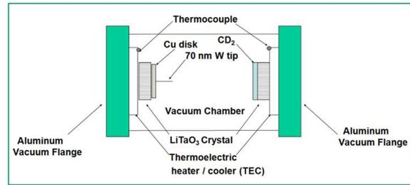
**FIGURE 2.** A diagram illustrating the experimental setup inside the vacuum chamber for the two-crystal pyroelectric accelerator at West Point.
