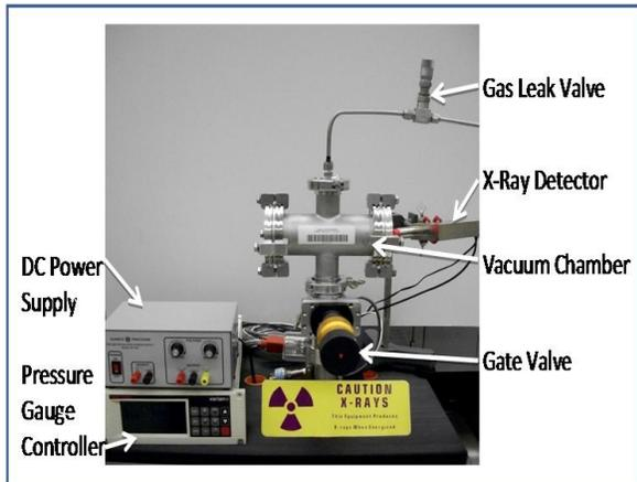
**FIGURE 1.** A picture of the experimental setup with associated diagnostics and power supply. The gas leak valve is not used until  $D_2$  gas is added to the system. In the experiments presented here, Bremsstrahlung x-rays were generated by the ionization and acceleration of residual gas particles in the vacuum system.
